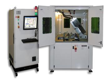
clamshell moves to the next solder location and the wire carrier to the next sensor. After each laser soldering is completed, a second CCD captures an image of the solder joints.
