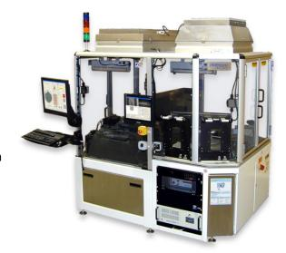
software computes wafer-to-table orientation before the wafer moves to the trench inspection sequence. Here, the Micro-Epsilon profilometer inspects three-dimensional features of the wafer, providing final resolutions of less than 0.1 micron. The robot transfers the inspected wafer back to its original slot in the appropriate cassette and continues processing additional wafers in each cassette.
