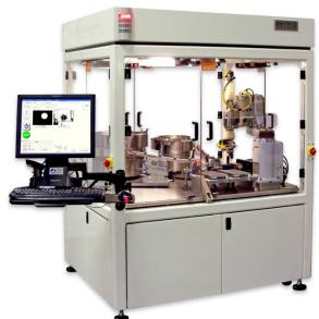
The automated, recipe-driven process allows for user input and real-time process monitoring, though operator attention is required only to maintain bulk part supplies and remove completed trays.
