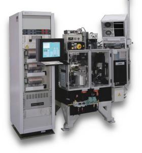
Waferbot transfers the completed wafer A to a temporary storage slot before moving wafer B to the wafer chuck for alignment, inspection, and glue application. Waferbot then transfers wafer A from the storage slot to the unload cassette and repeats the process for all remaining wafers.
