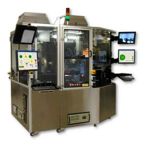
quill assembly picks up and holds the plate in position while the wafer aligns to the nozzle plate. The quill then moves the plate downward against the wafer and narrow UV light beams tack the plate to the wafer. The robot transfers the completed wafer to the UV-flood station, where intense UV light cures the adhesive to complete the nozzle-to-wafer bond.
