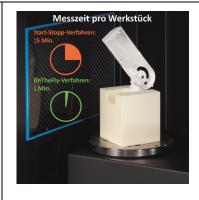
Measuring an inhaler: measurement time for start-stop and OnTheFly methods
